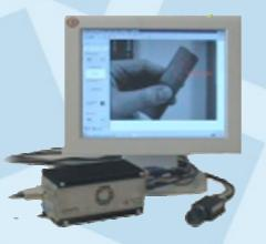
As a standard solution, PATTERN EXPERT offers a system which additionally includes a compact industry PC ("LVmPC") and a progressive scan camera from Leutron Vision. The standard system is shown in the image.
